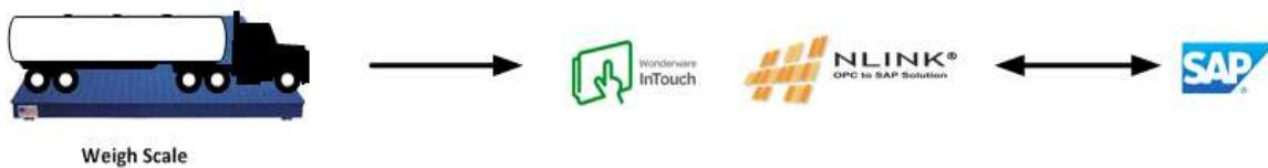
Once the destination is confirmed and the carrier validated, the operators are then allowed to enter the actual desired quantity of goods to be loaded and the loading starts. Once the loading is complete, the final (actual) loaded quantity information is gathered, (via an automated weighing scale), and sent to SAP. SAP verifies that all the information is correct and generates a bill of lading (BOL), and any other necessary documents, for the driver.
